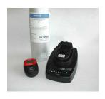
Periodically, simple proper operation of the **ECOTOX** gas detector can be checked by the optional **GAS TESTSTATION**. The unit performs a bump test that takes about  $15 \sim 30$  seconds. During the test operation and functionality of the **ECOTOX** detector
